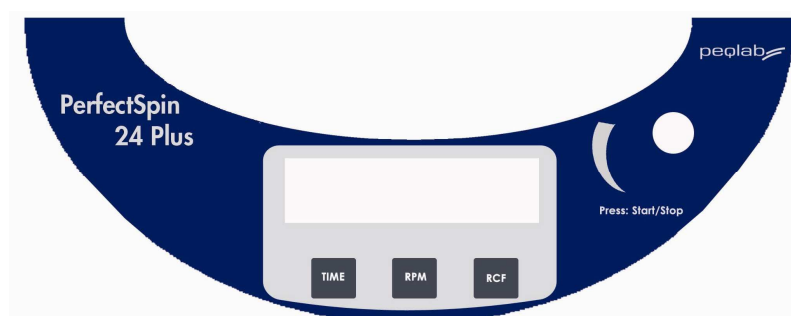
Figure 2: PerfectSpin 24 Plus control panel layout
