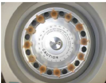
Figure 1: Loading the rotor to achieve balance
